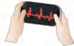
Patient initiated (or medical professional) intermittent ECG rhythm strip using smartphone or dedicated connectable device
